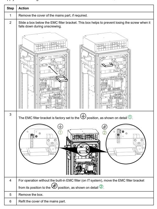
**NOTE:** Do not operate the module with the EMC filter bracket removed.
