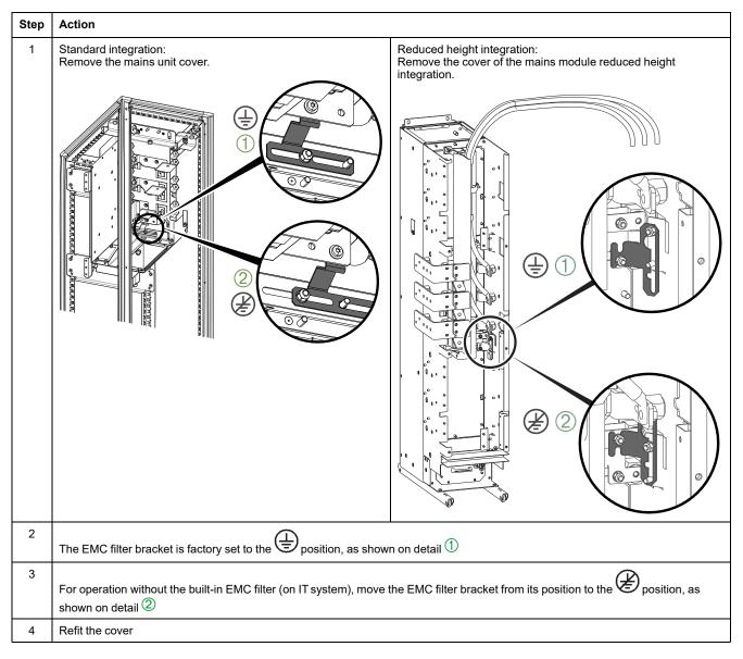
**NOTE:** Do not operate the module with the EMC filter bracket removed.
