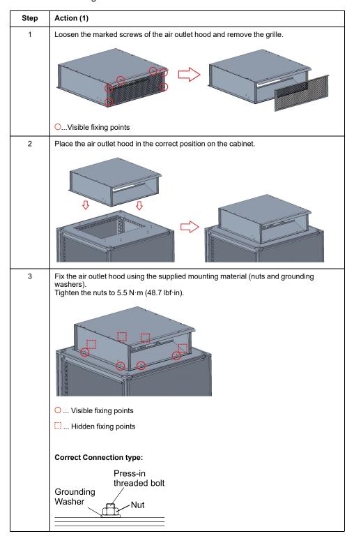
Drive Systems Mechanical Installation
