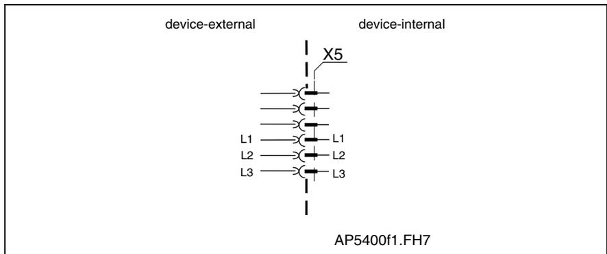
Fig. 5-58: Three-phase mains connection
