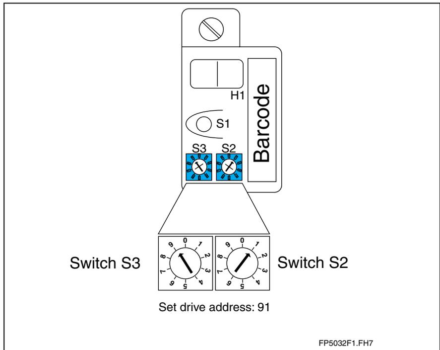
Fig. 5-71: Setting the drive address using a decade switch
