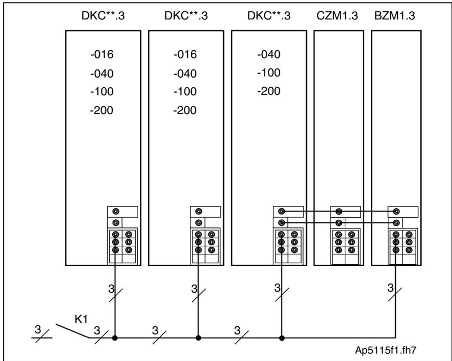
Fig. 4-23: Group supply without DC bus connection
