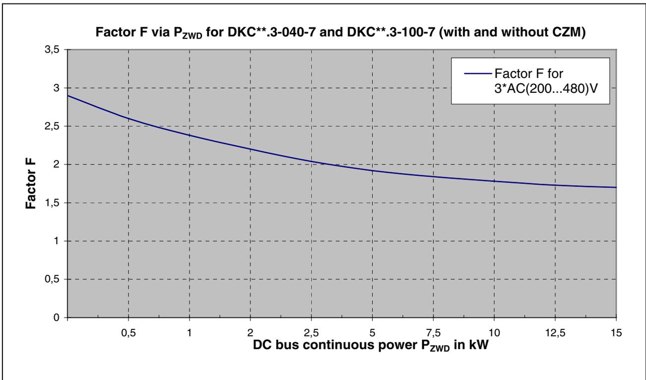
Fig. 11-9: Connected load factor for DKC\*\*.3-040-7 and DKC\*\*.3-100-7
