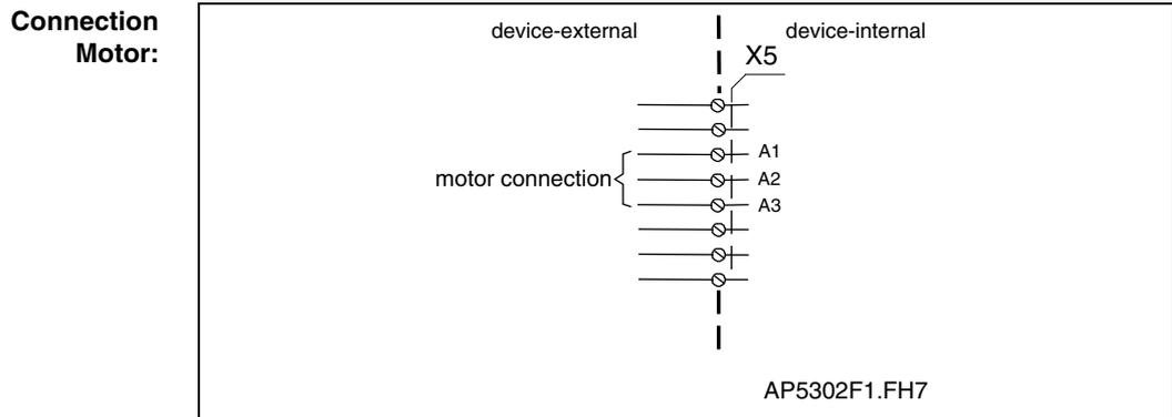
Fig. 4-94: Motor connections
