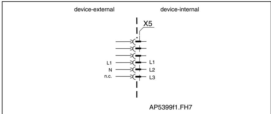
Fig. 5-57: Single-phase mains connection
