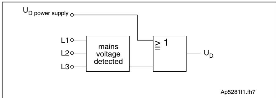
Fig. 4-148: Correlation of U<sub>D</sub> power supply and U<sub>D</sub> (U<sub>D</sub> message)
