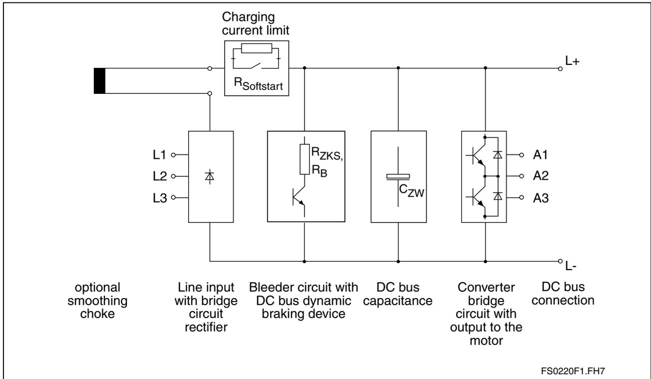
Fig. 4-10: Block diagram of the DKC\*\*.3-200-7-FW power section
