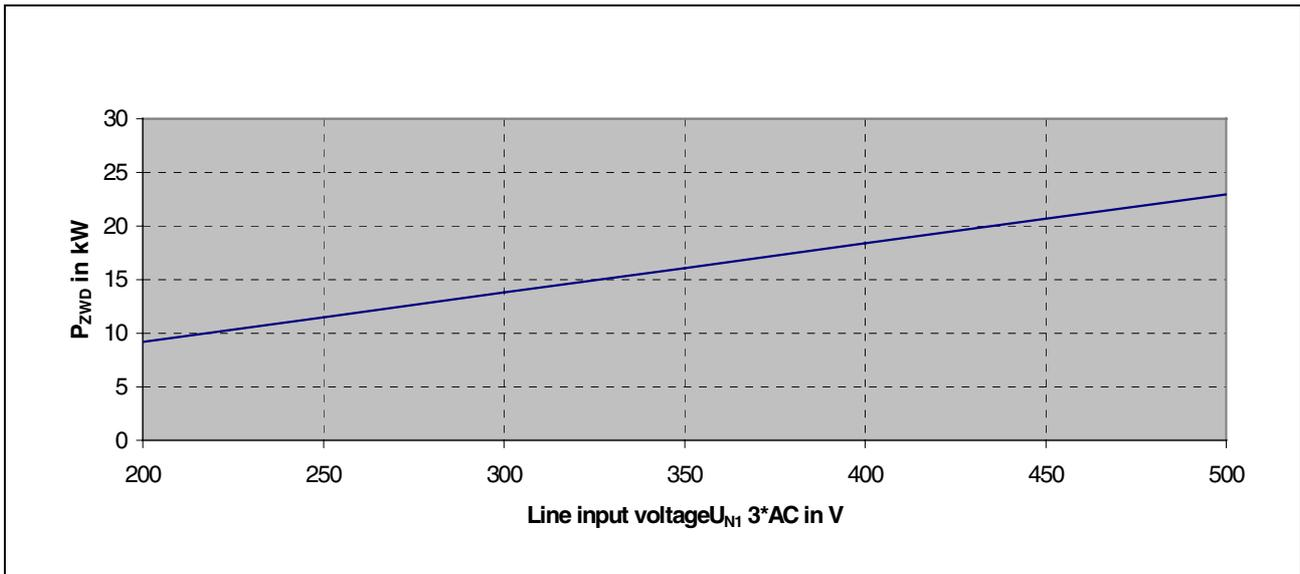
Fig. 4-34: Allowed DC bus continuous power for Single source supply
