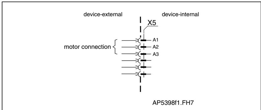
Fig. 5-55: Motor connections
