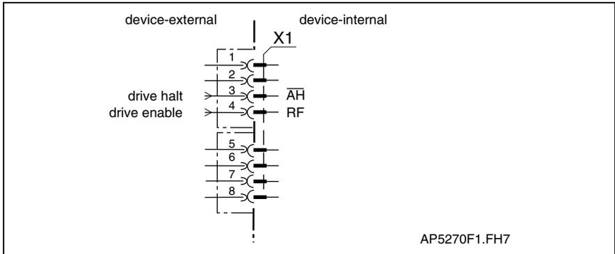
Fig. 4-53: Connections for drive halt and drive enable
