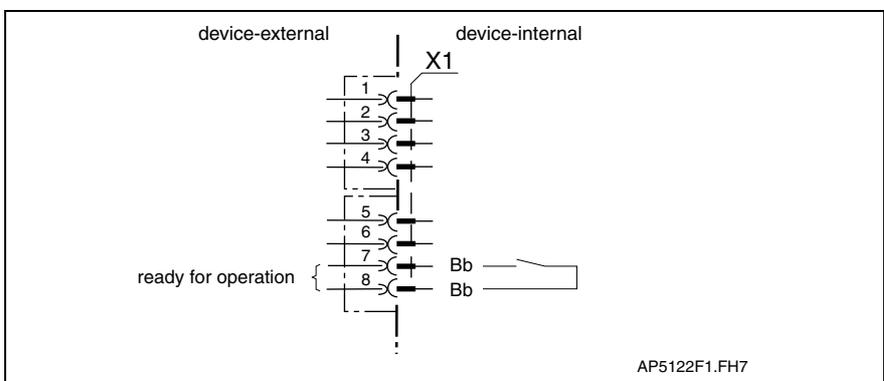
Fig. 6-16: Connections for ready to operate contact
