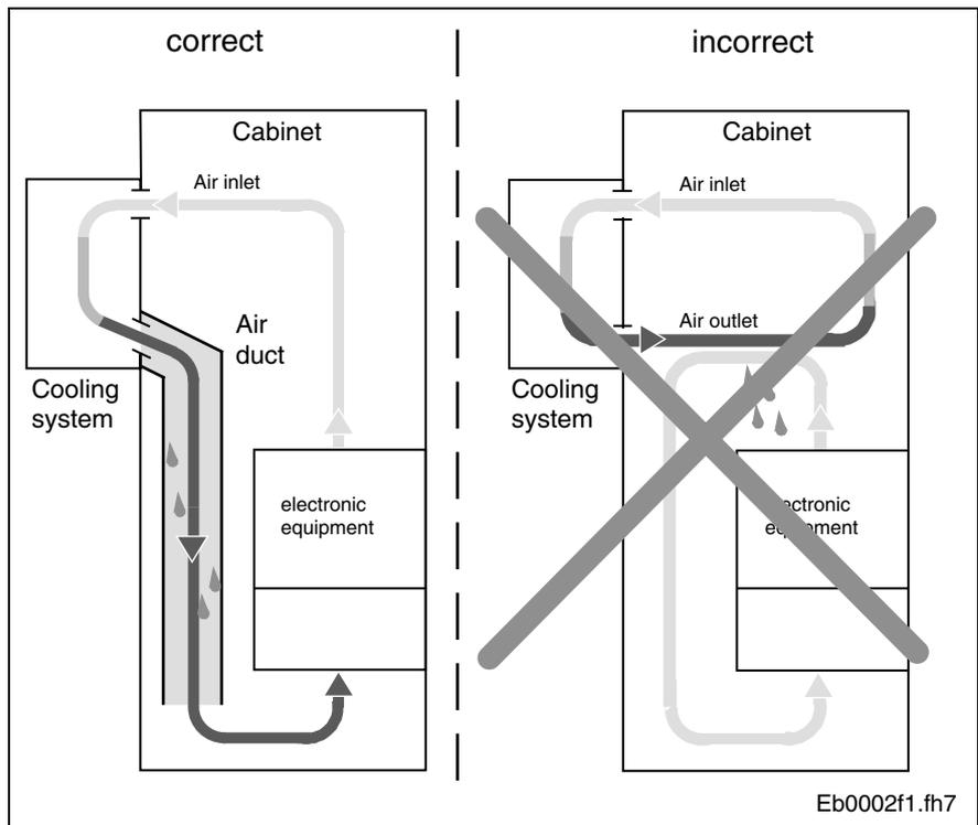
Fig. 12-20: Arranging cooling unit on front of cabinet
