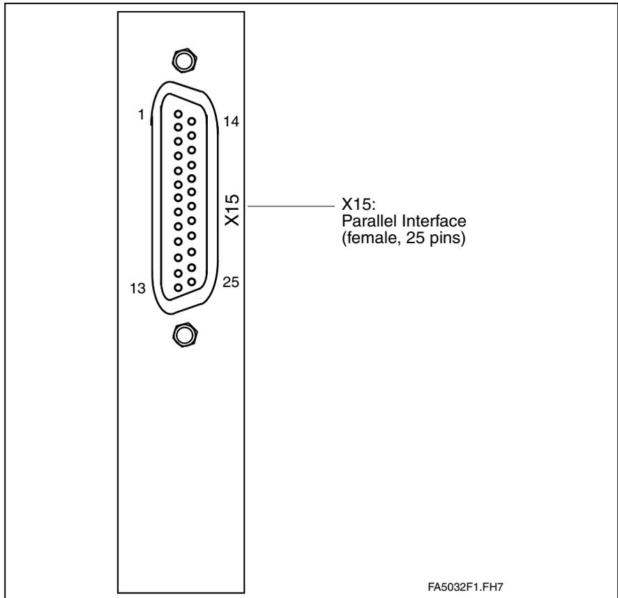
Fig. 4-159: View of interface to command communications
