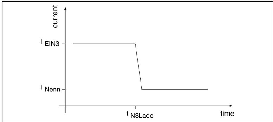
Fig. 5-6: Charging current profile of control voltage
