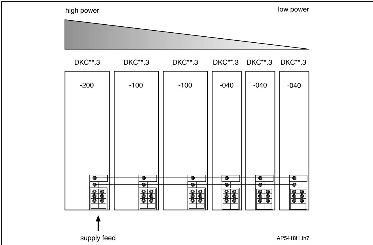
Fig. 12-18: Example of arrangement of a "Central feed"
