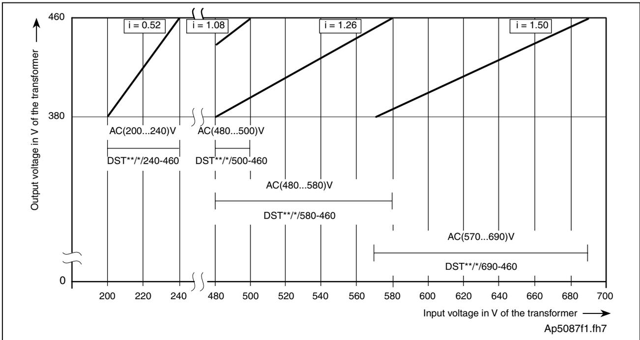
Fig. 10-1: Classification of three-phase autotransformers in rating groups
