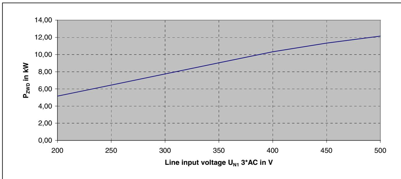
Fig. 4-33: Allowed DC bus continuous power for Single source supply
