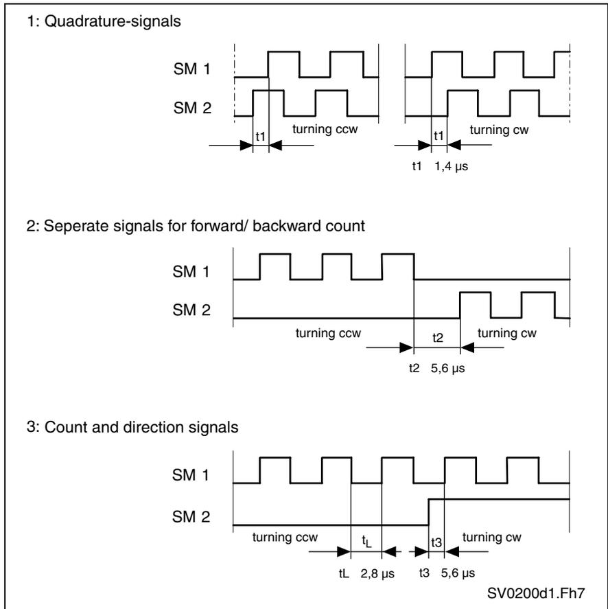
Fig. 4-174: Stepper motor interface types of control
