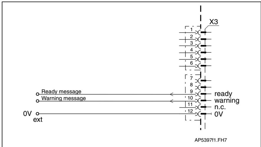
Fig. 5-41: Control outputs
