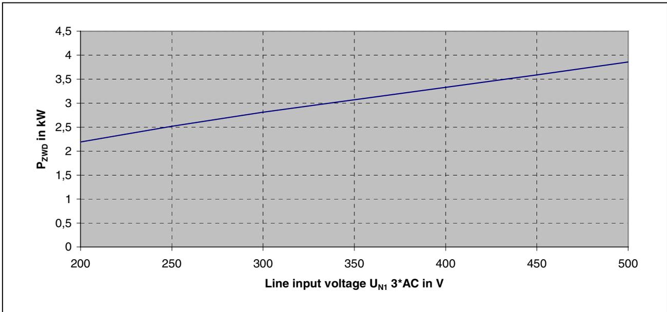
Fig. 4-31: Allowed DC bus continuous power for Single source supply
