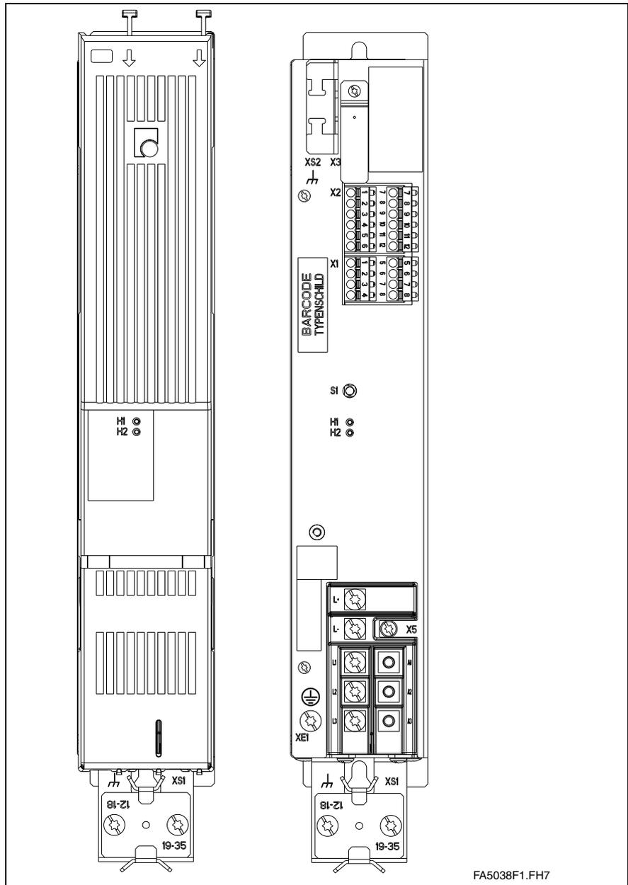
Fig. 6-8: Front view Auxiliary Bleeder Module BZM01.3
