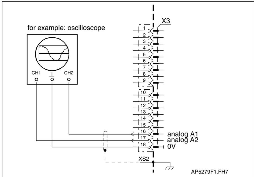
Fig. 4-79: Connection example of outputs A1 and A2
