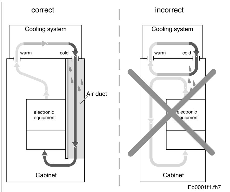
Fig. 12-19: Arranging cooling unit on cabinet
