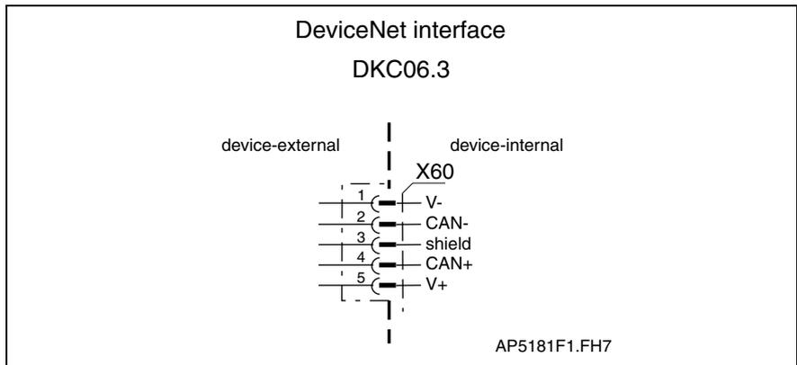
Fig. 4-207: DeviceNet Interface for DKC06.3
