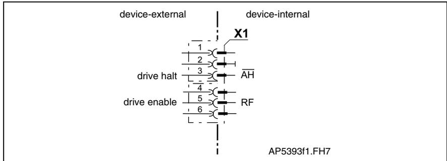
Fig. 5-26: Connections for drive halt and drive enable
