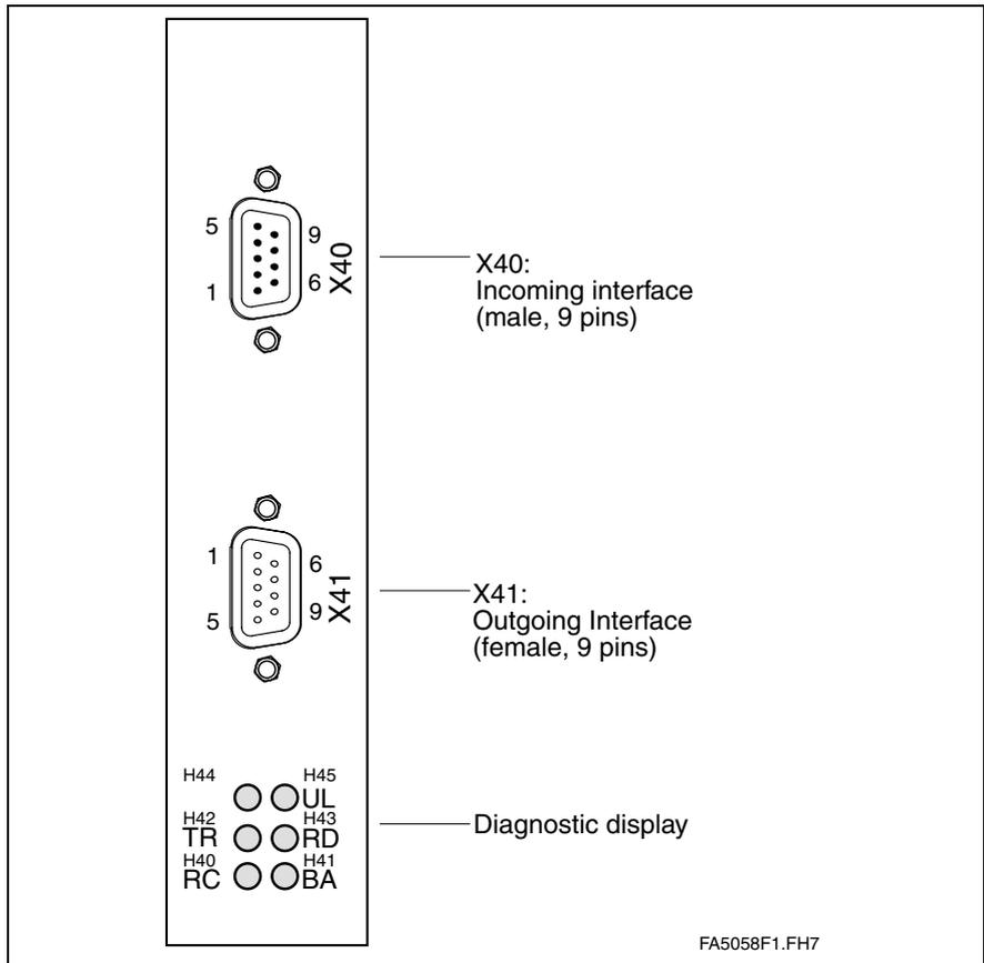
Fig. 4-193: View of command communication interface
