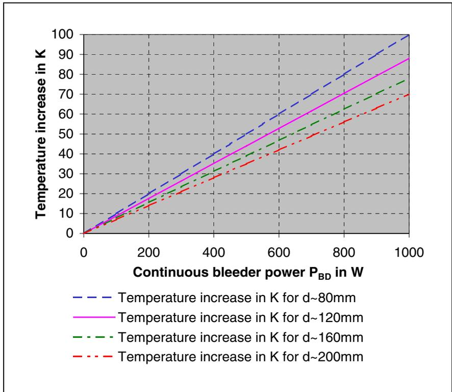
Fig. 12-14: Temperature increase DKC\*\*.3-200-7-FW
