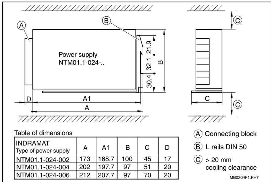
Fig. 9-2: Dimensional sheet DC24V – NTM power supplies
