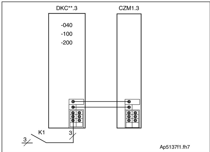
Fig. 7-13: Connection of auxiliary capacitance module CZM01.3
