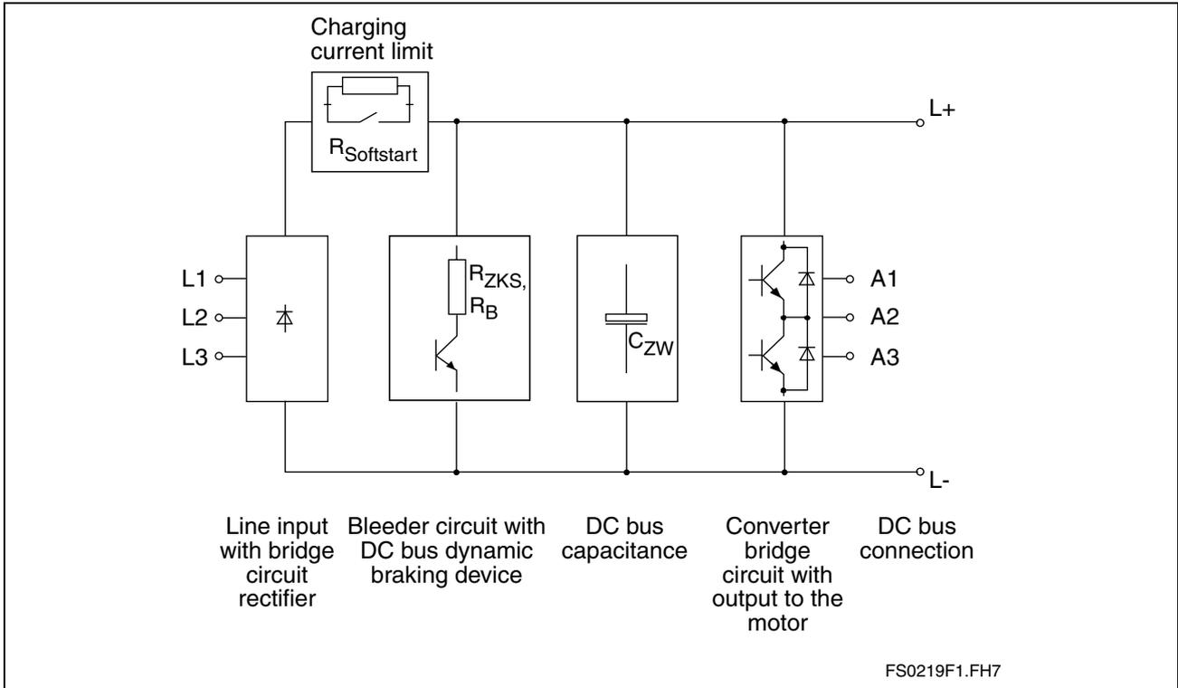
Fig. 4-9: Block diagram of the DKC\*\*.3-100-7-FW power section
