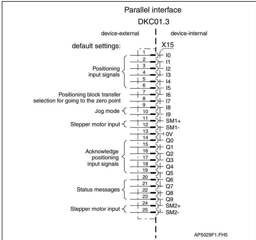
Fig. 4-162: Parallel interface for DKC01.3
