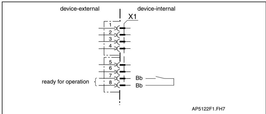
Fig. 4-56: Connections for ready to operate contact
