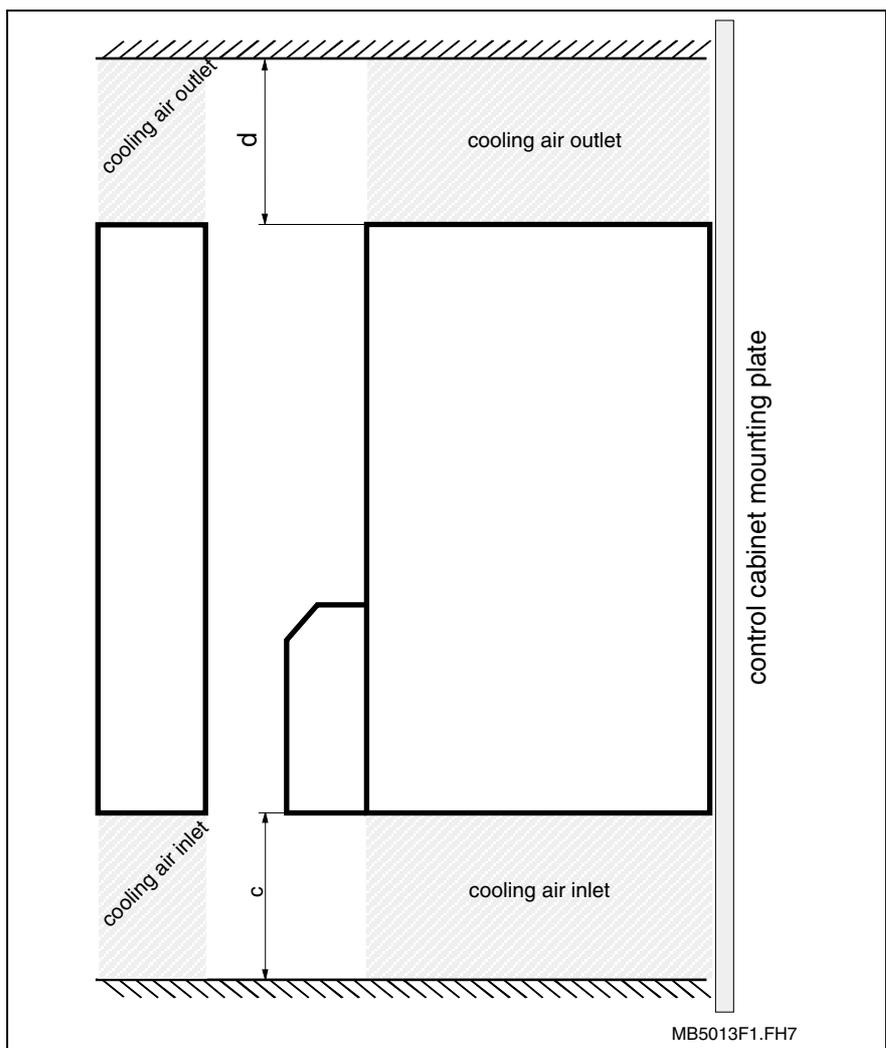
Fig. 12-10: Exit and entrance of cooling air
