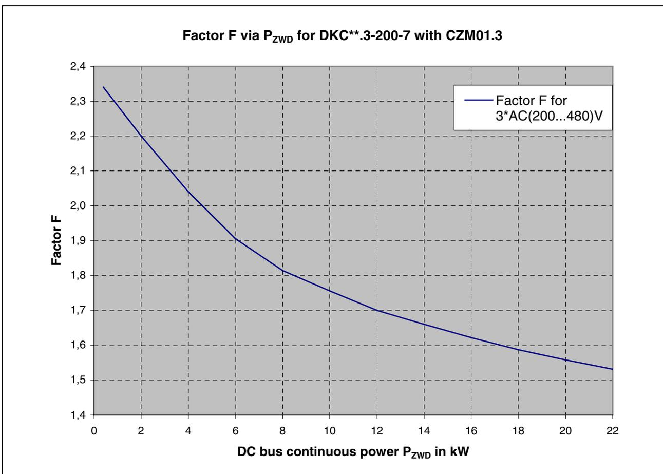
Fig. 11-11: Connected load factor for DKC\*\*.3-200-7 with CZM01.3
