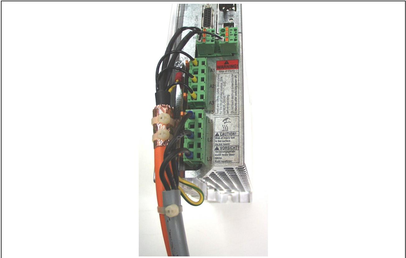
Fig. 16-27: Connection of motor and mains cable
