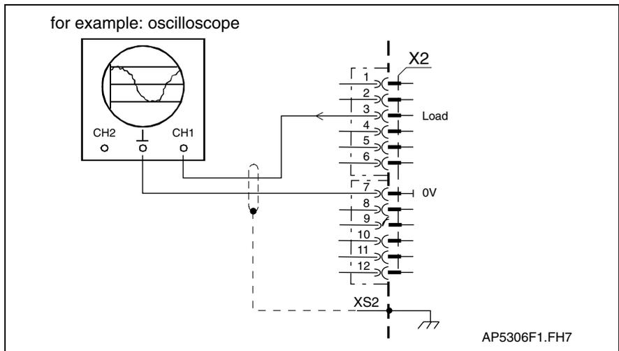
Fig. 6-26: Output load
