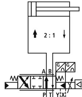
**Flow in mid position, “leakage oil pressure relief”**
