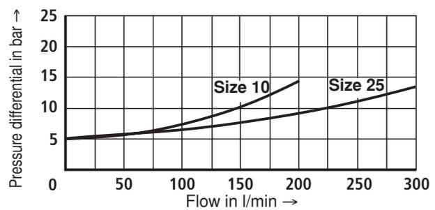
**Characteristic curves** (measured with HLP46,  $\vartheta_{oil} = 40 \text{ }^\circ\text{C} \pm 5 \text{ }^\circ\text{C}$  and amplifier VT VSPA1-11-1X, 1600 mA coil...)
