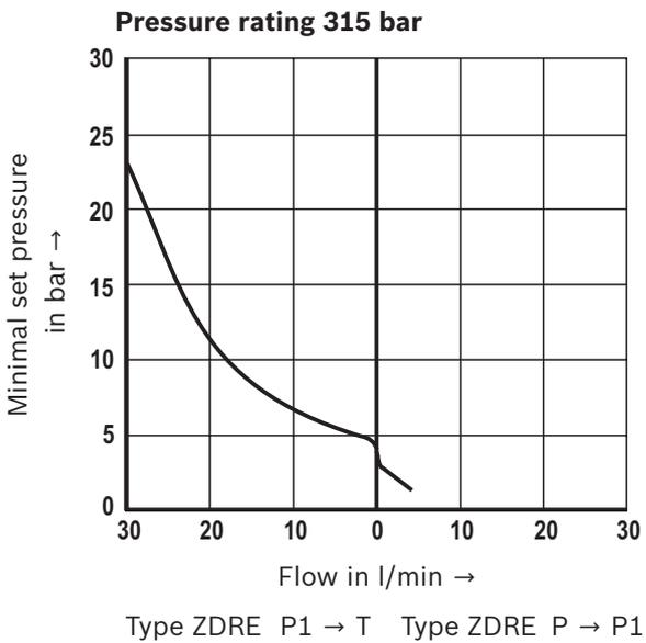
**Characteristic curves** (measured with HLP46,  $\vartheta_{oil} = 40 \text{ }^\circ\text{C} \pm 5 \text{ }^\circ\text{C}$ )
