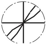
Zero point passage depending on manufacturing tolerance
