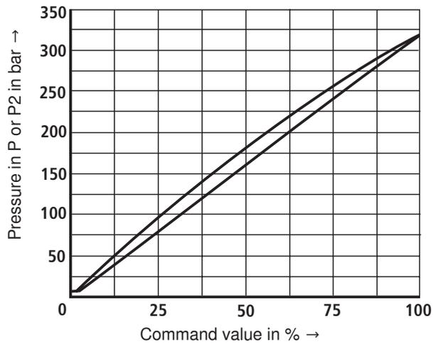
Pressure rating 350 bar ("y" external and internal)
