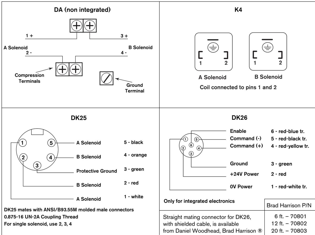
Terminal Connections and Block Diagram - 4 WRAE B 6...-1X/G24 N9 DK26 (K31) (DA)
