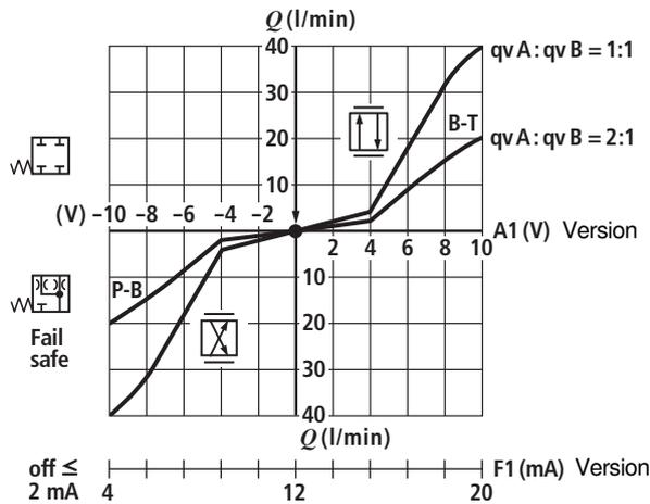
**Characteristic curves** (measured with HLP 46,  $\vartheta_{oil} = 40\text{ }^\circ\text{C} \pm 5\text{ }^\circ\text{C}$ )
