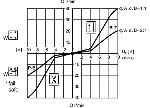
\*Fail-safe when enabling is not released.
