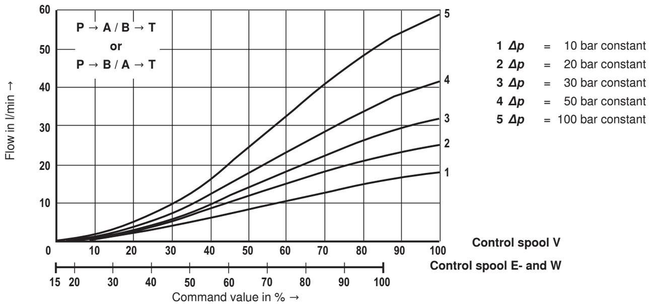
**32 l/min rated flow with 10 bar valve pressure differential**
