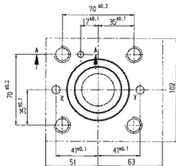
Installation dimensions DIN 24342, ISO/DIS 7368 (in mm)
