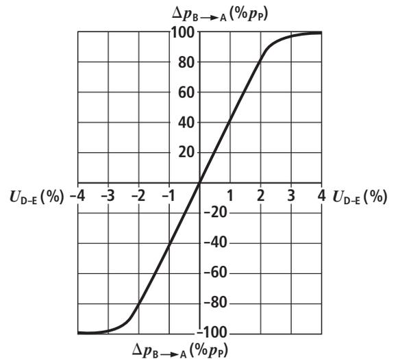
**Characteristic curves** (measured with HLP 46,  $\vartheta_{oil} = 40\text{ °C} \pm 5\text{ °C}$ )
