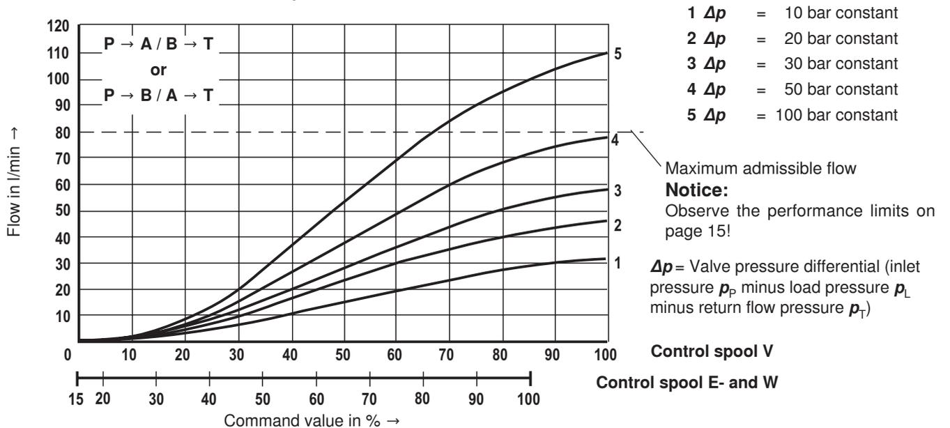
**Characteristic curves: Type 4WREE (measured with HLP46,  $\vartheta_{Oil} = 40 \text{ }^\circ\text{C} \pm 5 \text{ }^\circ\text{C}$  and  $p = 100 \text{ bar}$ ) Size 10**
