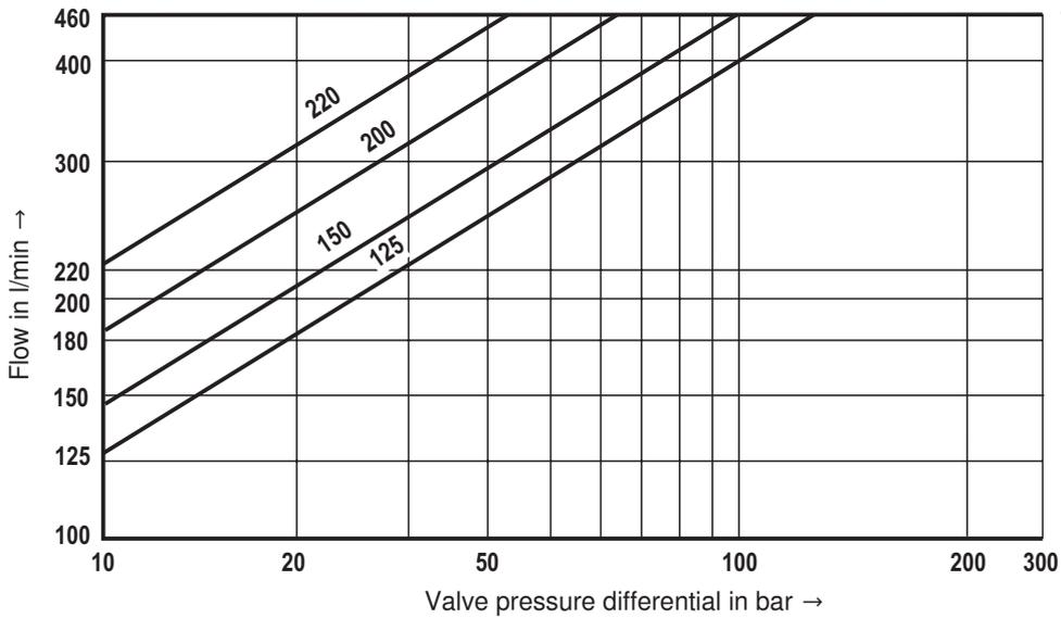
**1** = Recommended flow limitation (flow velocity 30 m/s) in the valve connection bores
