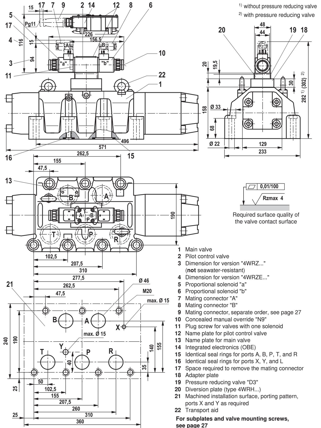
**Dimensions:** Flange connection size 52 (dimensions in mm)
