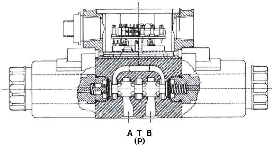
Proportional directional control valves Model 4 WRA B 6 and 4 WRAE B 6 are direct operated spool valves. They control the direction and quantity of flow to an actuator, for smooth acceleration to a desired velocity. The valve is normally operated by integrated electronics or a suitable amplifier. The 4 WRA B can be operated as a switching valve if proportional control is not required.
