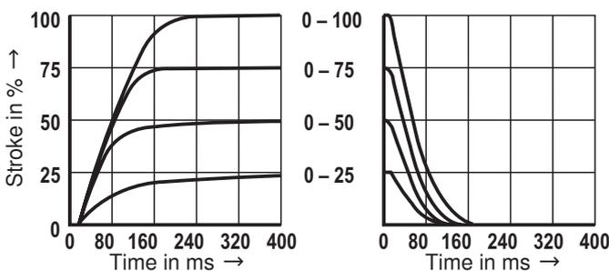
**Characteristic curves size 52** (control spool "E, W6-, EA, W6A" as well as HLP46,  $\vartheta_{oil} = 40 \text{ }^\circ\text{C} \pm 5 \text{ }^\circ\text{C}$  and  $p = 100 \text{ bar}$ )
