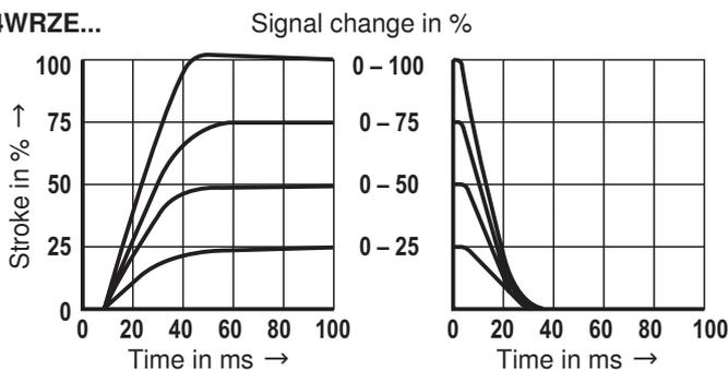
**Characteristic curves size 16** (control spool "E, W6-, EA, W6A" as well as HLP46,  $\vartheta_{oil} = 40 \text{ }^\circ\text{C} \pm 5 \text{ }^\circ\text{C}$  and  $p = 100 \text{ bar}$ )
