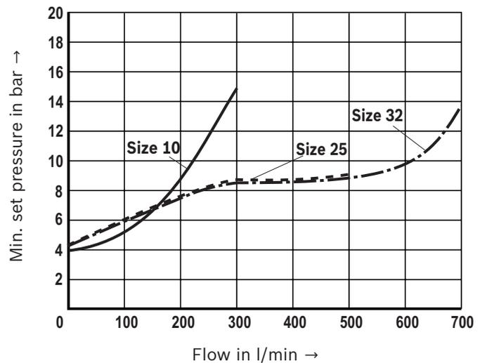
The characteristic curves apply to output pressure in T or Y = 0 bar in the total flow range.
