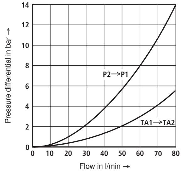
**Characteristic curves** (measured with HLP46,  $\vartheta_{oil} = 40 \text{ }^\circ\text{C} \pm 5 \text{ }^\circ\text{C}$ )
