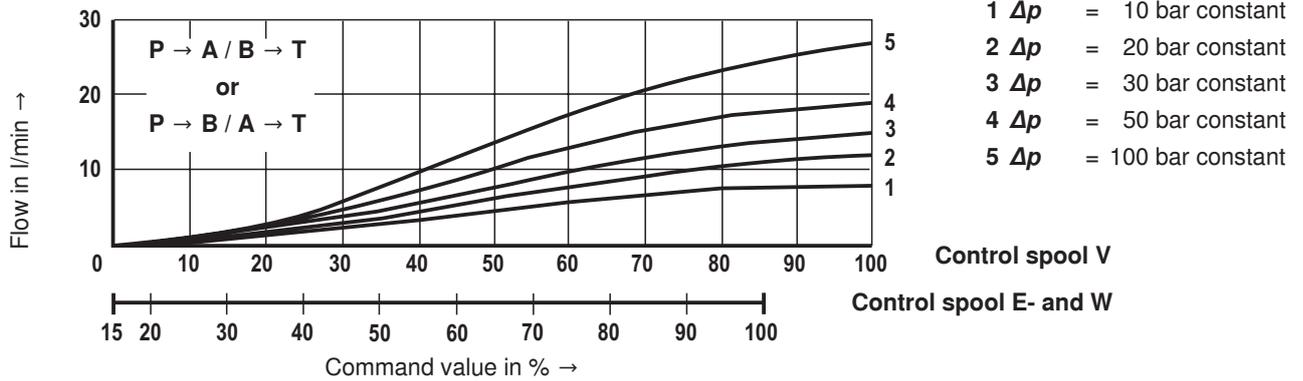
**16 l/min rated flow with 10 bar valve pressure differential**
