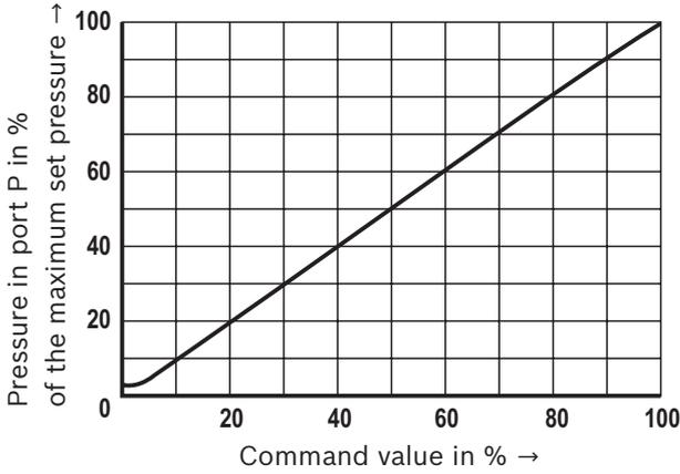
**Minimum set pressure in port P with command value 0 V and/or 4 mA depending on the flow**
