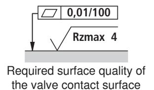
**Tolerances according to:** – General tolerances ISO 2768-mK
