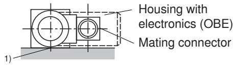
The mating connector can be brought to the desired position after the nut was loosened (see page 17, 18).
