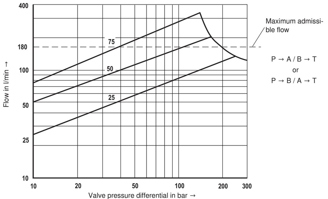
Observe the maximum admissible flow of 180 l/min!
