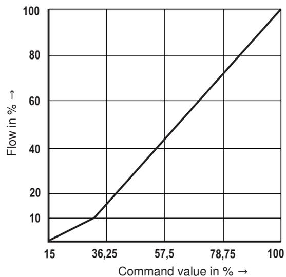
**Characteristic curves: Size 10 (measured with HLP46,  $\vartheta_{oil} = 40 \text{ }^\circ\text{C} \pm 5 \text{ }^\circ\text{C}$ )**
