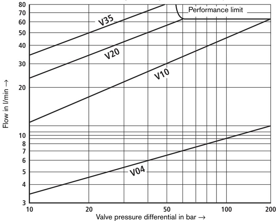
**Characteristic curves of size 10 (measured with HLP46,  $\vartheta_{oil} = 40\text{ °C} \pm 5\text{ °C}$ )**
