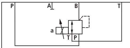
Example of valve with integrated control electronics
