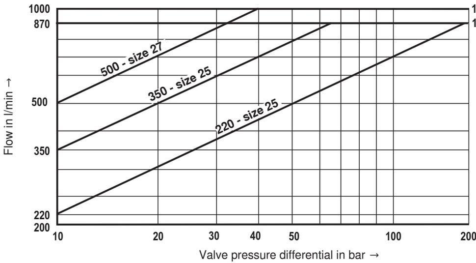
1 = Recommended flow limitation (flow velocity 30 m/s) in the valve connection bores
