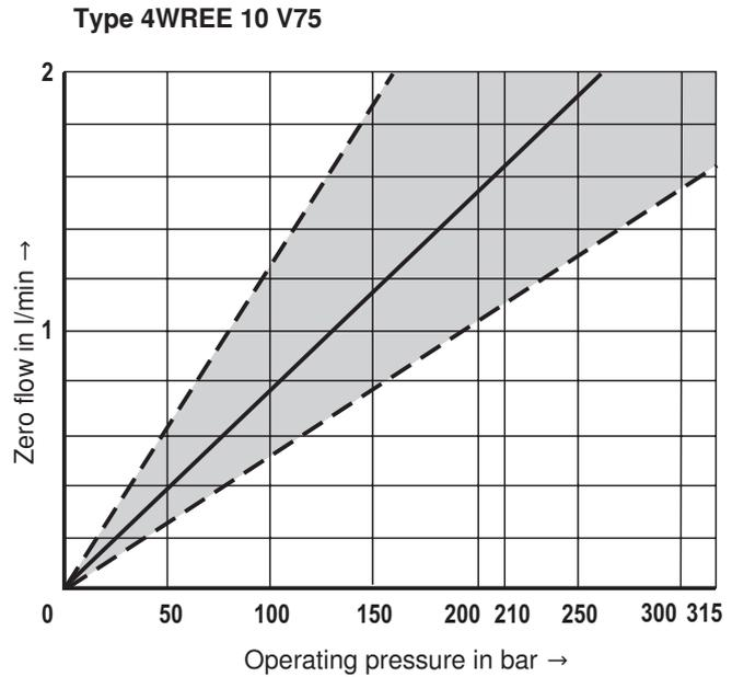
**Characteristic curves: Type 4WREE (measured with HLP46,  $\vartheta_{Oil} = 40 \text{ }^\circ\text{C} \pm 5 \text{ }^\circ\text{C}$  and  $p = 100 \text{ bar}$ ) Size 6**
