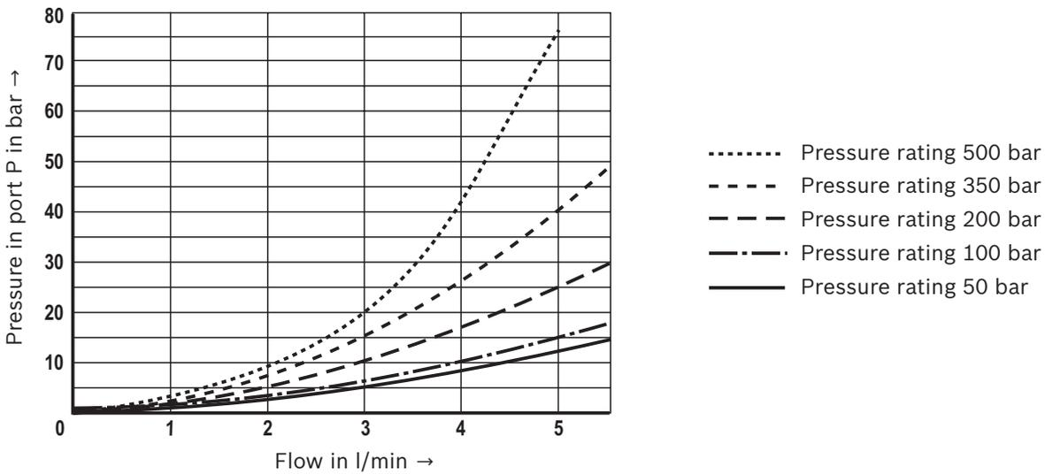
**Pressure in port P depending on the flow** (applies to all pressure ratings)
