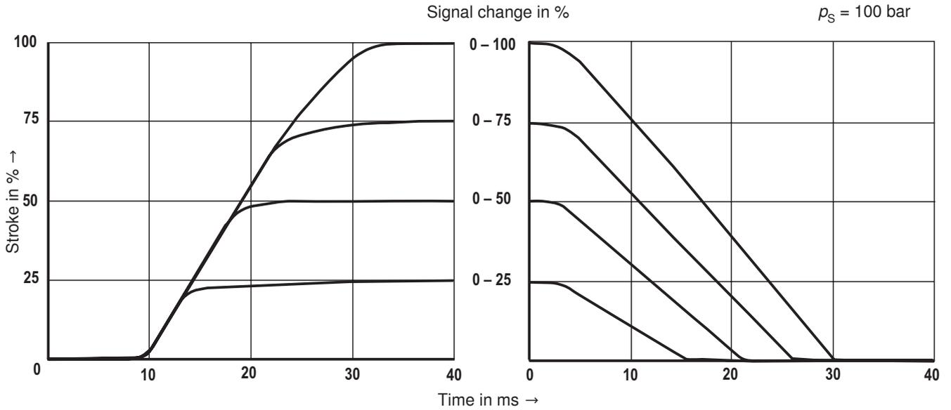
**Flow/load function with maximum valve opening**
