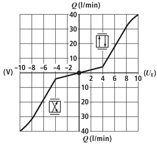
**Characteristic curves** (measured with HLP 46,  $\vartheta_{oil} = 40 \text{ }^\circ\text{C} \pm 5 \text{ }^\circ\text{C}$ )
