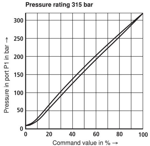
**Characteristic curves** (measured with HLP46,  $\vartheta_{\text{oil}} = 40 \text{ °C} \pm 5 \text{ °C}$ )**Pressure differential in dependence upon the flow**
