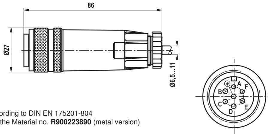
Mating connector according to DIN EN 175201-804
