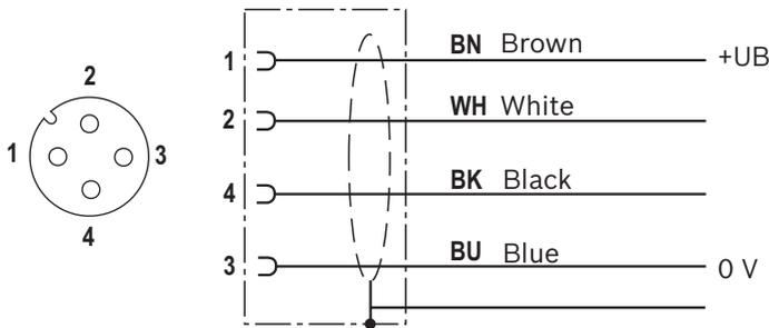
**The connection for the protective earthing conductor is not provided**
