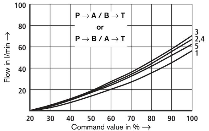
$\Delta p =$  Valve pressure differential (inlet pressure  $p_p$  minus load pressure  $p_L$  and minus return pressure  $p_T$ )
