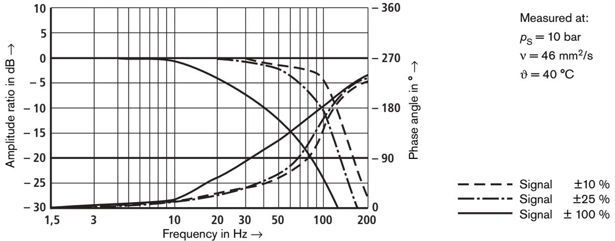
**Flow/load function at max. valve aperture (tolerance  $\pm 10\%$ )**
