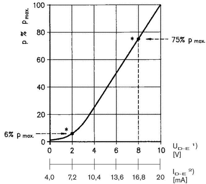
Pressure in port A as a function of the main stage nominal flow rate
