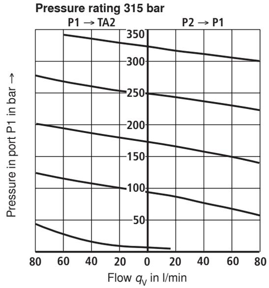
Min. set pressure in dependence upon the flow at zero command value
