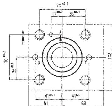
Installation dimensions DIN 24342, ISO/DIS 7368 (nominal dimensions in mm)
