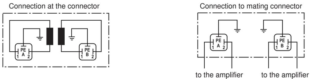
**For type .WRZ...** (for external electronics – with version "J" = seawater-resistant)
