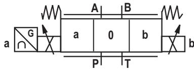
**Proportional directional valve with integrated electronics**
