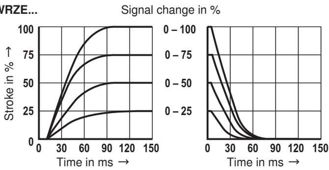
**Characteristic curves size 25** (control spool "E, W6-, EA, W6A" as well as HLP46,  $\vartheta_{oil} = 40 \text{ }^\circ\text{C} \pm 5 \text{ }^\circ\text{C}$  and  $p = 100 \text{ bar}$ )
