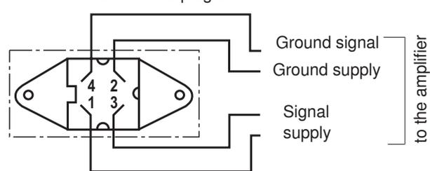
Mating connector 4-pole Pg7-G4W1F separate order under the Material no. **R900023126**
