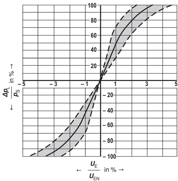
**Characteristic curves: Type 4WREE (measured with HLP46,  $\vartheta_{Oil} = 40 \text{ }^\circ\text{C} \pm 5 \text{ }^\circ\text{C}$ ) Size 6 and 10**
