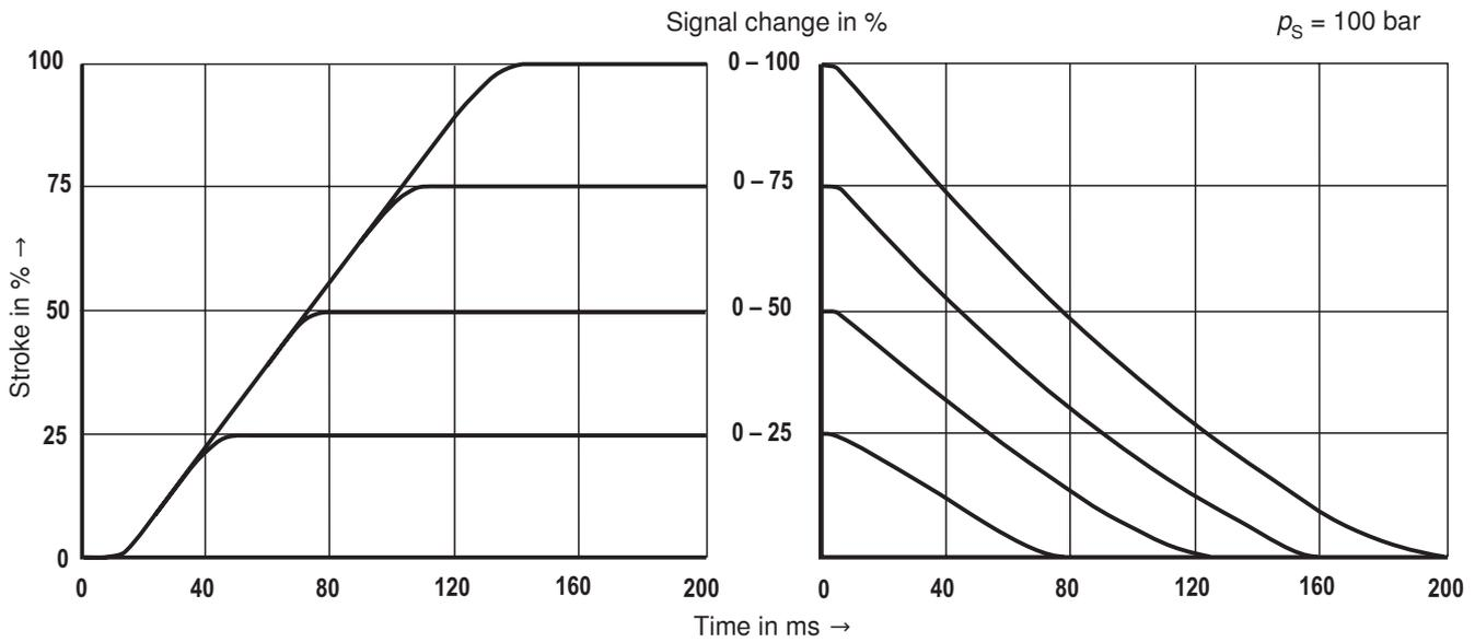
**Flow/load function with maximum valve opening**
