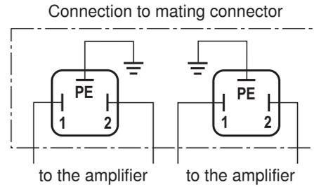
Mating connector CECC 75 301-803-A002FA-H3D08-G according to DIN EN 175301-803 and ISO 4400
