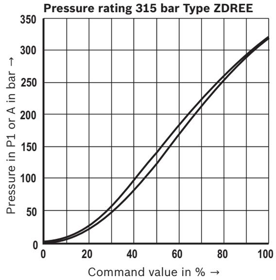
**Characteristic curves** (measured with HLP46,  $\vartheta_{oil} = 40 \text{ °C} \pm 5 \text{ °C}$ )
