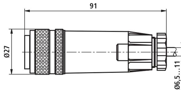
Plug-in connector to DIN EN 175201-804
