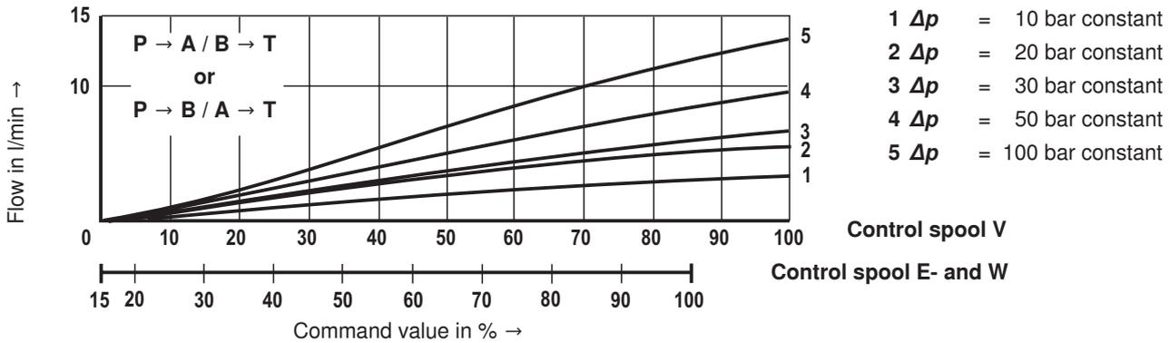
**Characteristic curves: Type 4WREE (measured with HLP46,  $\vartheta_{Oil} = 40 \text{ }^\circ\text{C} \pm 5 \text{ }^\circ\text{C}$  and  $p = 100 \text{ bar}$ ) Size 6**
