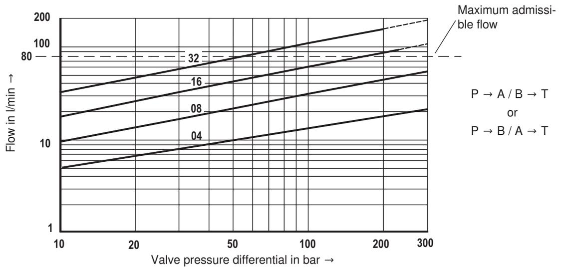
Observe the maximum admissible flow of 80 l/min!
