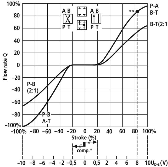
**Control spool with asymmetric metering notches**
