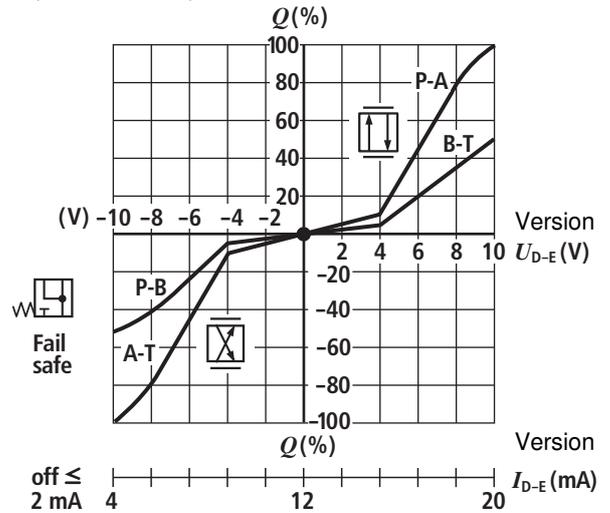
**Characteristic curves** (measured with HLP 46,  $\vartheta_{oil} = 40 \text{ }^\circ\text{C} \pm 5 \text{ }^\circ\text{C}$ )
