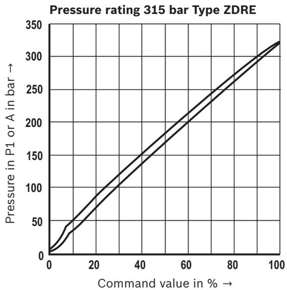
**Characteristic curves: Type (Z)DREE** (measured with HLP46,  $\vartheta_{oil} = 40 \text{ °C} \pm 5 \text{ °C}$ )
