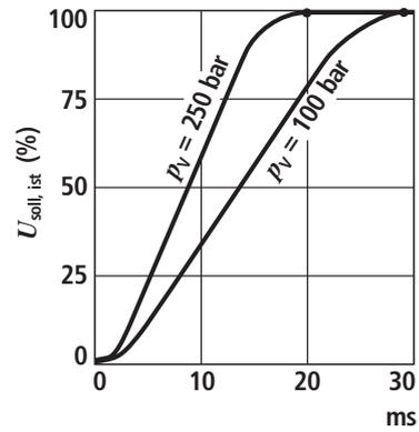
**Characteristic curves** (measured with HLP 46,  $\vartheta_{Oil} = 40 \text{ }^\circ\text{C} \pm 5 \text{ }^\circ\text{C}$ )
