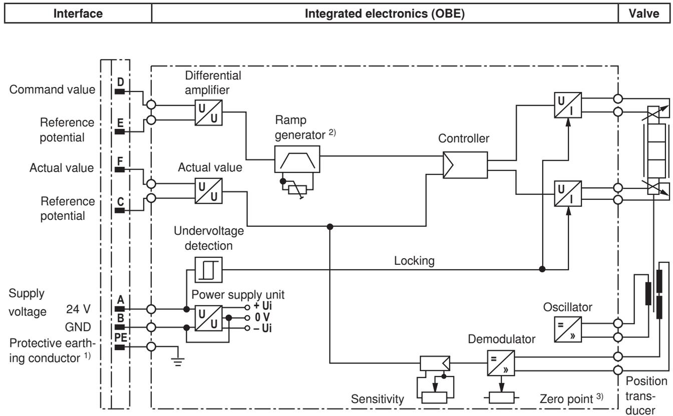
**Notice: Electric signals taken out via control electronics (e.g. actual value) must not be used for switching off safety-relevant machine functions!**
