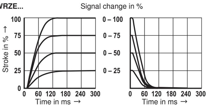
**Characteristic curves size 32** (control spool "E, W6-, EA, W6A" as well as HLP46,  $\vartheta_{oil} = 40\text{ }^\circ\text{C} \pm 5\text{ }^\circ\text{C}$  and  $p = 100\text{ bar}$ )
