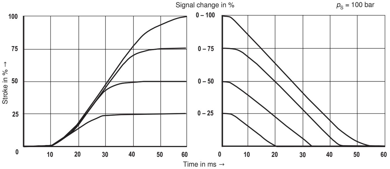
**Flow/load function with maximum valve opening**
